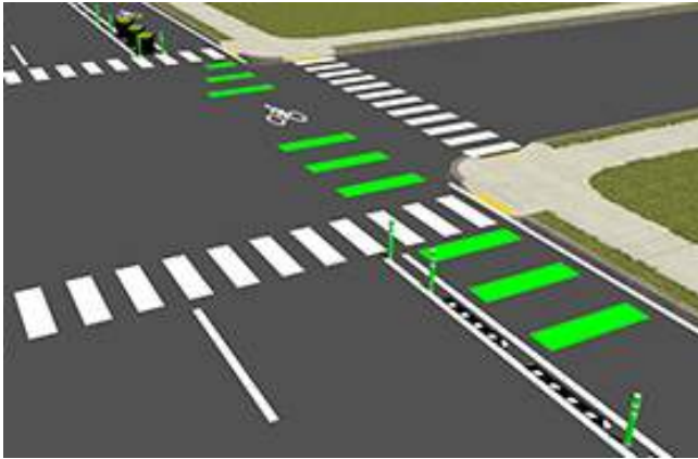
Wide, high visibility crosswalk markings with different color striping for pedestrians and bicyclists
