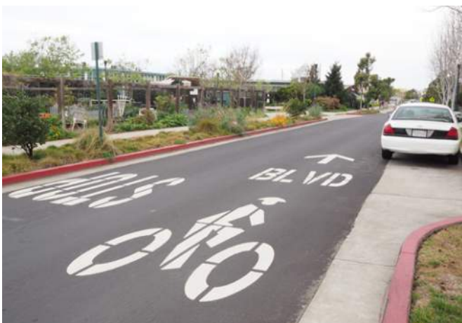
Bike Boulevard Sharrows with curb bump-outs for on-street parking
