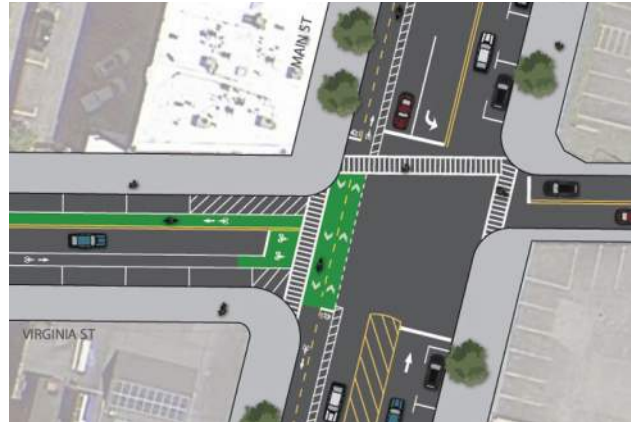
Painted bike lanes and bike boxes at intersection with white striping for pedestrian crossings
